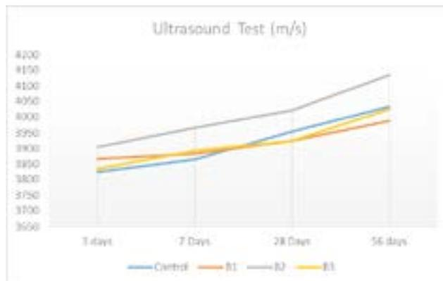
**Fig.4.** Ultrasonic pulse velocity values (m/s).
