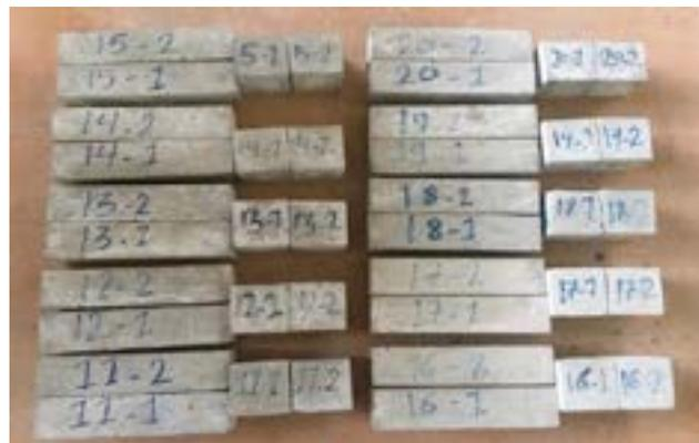
**Fig. 1.** The manufactured geopolymer samples
