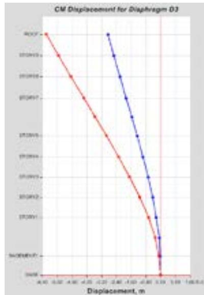
**Figure 8:** Center of mass displacement for diaphragm D3
