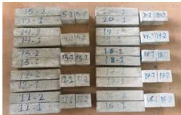
**Fig. 1.** The manufactured geopolymer samples
