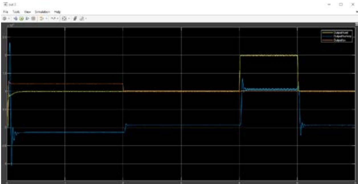
Above From the graph we can see charged battery is providing power to load and battery is charged by the renewable resources that is solar. Extra power is transferred to the grid sometimes it takes power from other sources. At starting the solar power is very less this is because of solar data i.e. irradiance data has small values at starting time.
