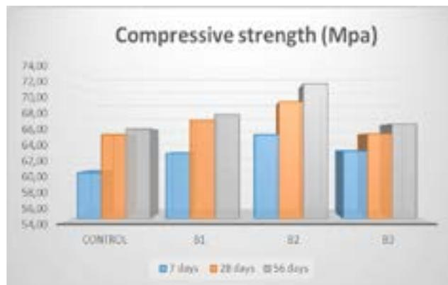
**Fig. 2.** The diagram of compressive strength for the manufactured samples
