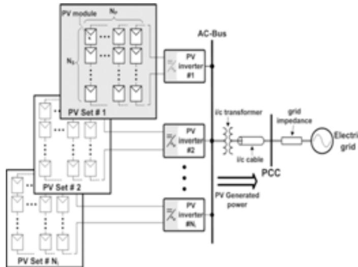
Fig.1 Block diagram of the large PV plant [31].
