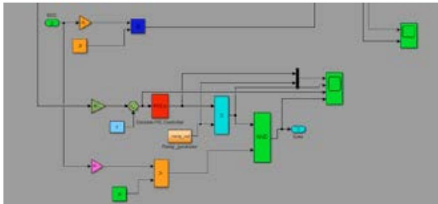
With the hybrid voltage and current mode control, the inverter is controlled as a current source to generate the reference power in the grid-tied mode. And its output power should be the sum of the power injected to the grid and the load demand  $P_{load} + jQ_{load}$ , which can be expressed as follows by assuming that the load is represented as a parallel RLC circuit:
