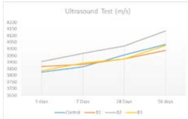
**Fig.4.** Ultrasonic pulse velocity values (m/s).
