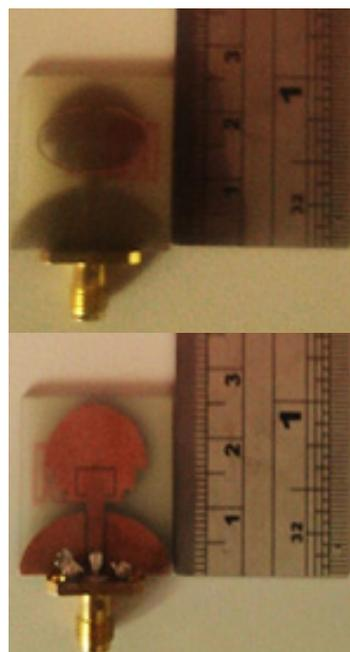
Fig. 8 photograph of fabricated antenna
