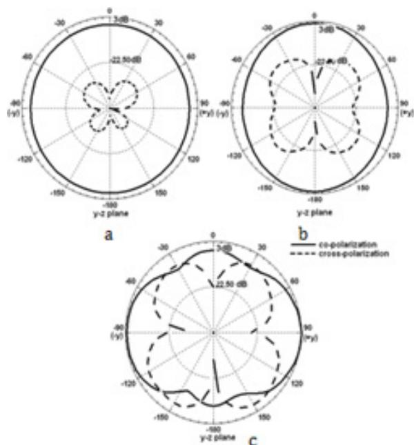
Fig. 6 measured radiation patterns of the proposed antenna for two planes at (a) 3.0 GHz, (b) 6.0 GHz and (c) 8.0 GHz
