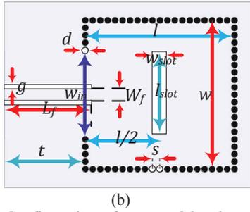
**Figure 1.** Configuration of proposed bandpass filter a) multilayered view b) cavity resonator with parameters ( $d=0.5$ ,  $s=0.6$ ,  $W_f=1$ ,  $g=0.3$ ,  $w=12$ ,  $l=12$ ,  $w_{slot}=.8$ ,  $l_{slot}=9$ ,  $L_f=7$ ,  $t=6$  and  $w_{in}=7.2$ ; all unit are mm)
